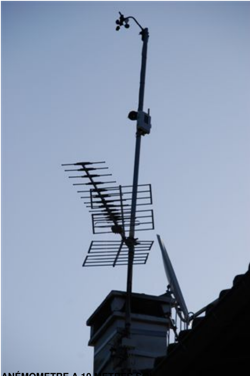
ANÉMOMETRE A 10 METRES SOL
